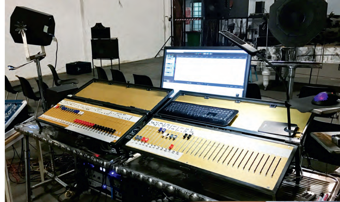
Abb. 16: The actual controller is version 3 made with an iron / aluminium construction.
